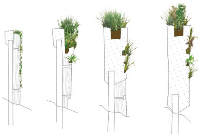
Different concepts for timbering arrangements for ecological and visual enhancement of near-vertical intertidal walls
